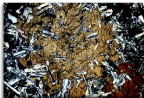
Figure 2. Microscope photo of ophitic basalt. Small light crystals are plagioclase feldspar. The large brownish crystals are augite. Field of view is about 2 mm
