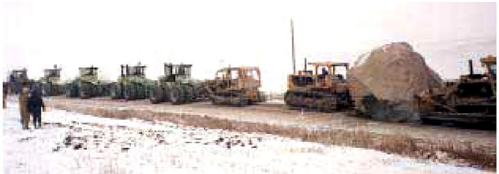
Seven Steiger 4x4s and two Caterpillars pull, and D-6 and D-8 Caterpillars push Slayton Rock down the road.
