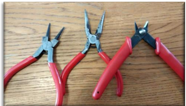
Round Nose Pliers, Needle Nose (or Long Nose) Pliers with teeth, and Wire Cutters,
